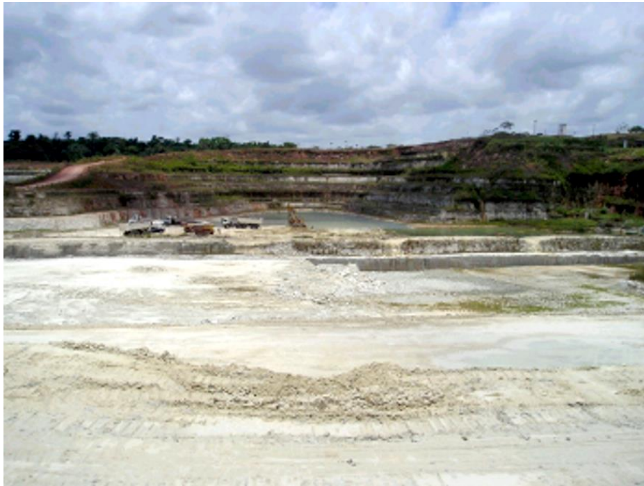
Figure 2 - General view of Mine B-17, showing part of the carbonatic section and sandstones (top, on the back). The pale gray levels correspond to different carbonatic lithofacies from the 20m section left.
