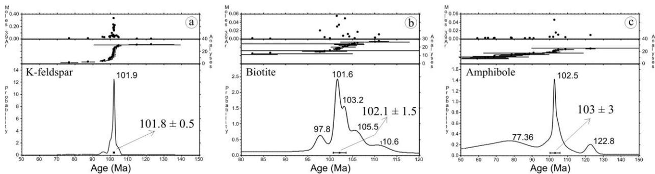
Figure 6 –  $^{40}\text{Ar}$ - $^{39}\text{Ar}$  ages ( $2\sigma$  deviation) for minerals of the Cabo de Santo Agostinho granite.
